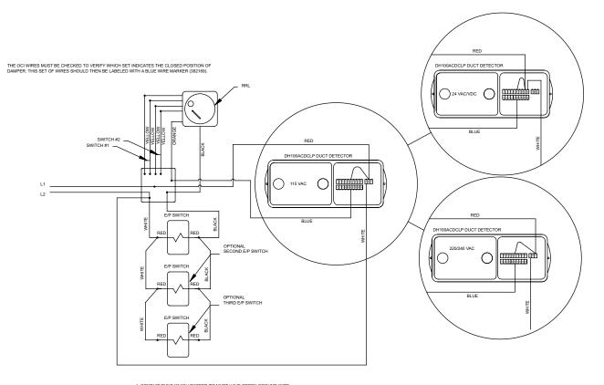
1. CONDUIT RUNS WHICH EXCEED 72" MUST HAVE GREEN GROUND WIRE. 2. FLEX CONDUIT MUST BE SECURED WITH A CONDUIT CLAMP (45226) WITHIN 12" OF CONDUIT TERMINATION AT THE HANDI-BOX OR ACTUATOR. CONDUIT RUNS MUST ALSO BE SECURED ALONG SLEEVE AT A MAXIMUM OF 24" ON CENTER.
